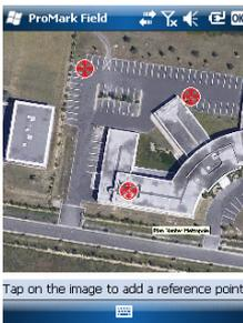
Georeferencing an image file means defining at least three reference points giving the position of the image in space.
